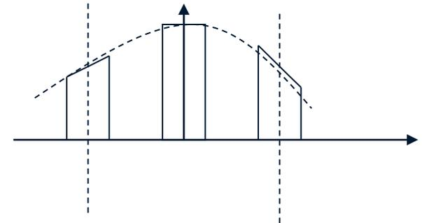
$$\varphi_{\text{PAM}}(\omega) = T/T_s \text{Sa}(\omega T/2) \sum_{n=-\infty}^{\infty} F(\omega - n\omega_s)$$
